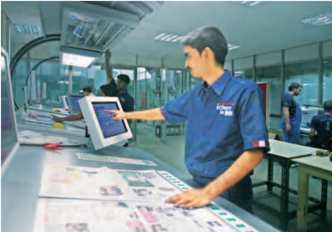
An operator adjusting the Console (control panel) of Regioman printing machine
